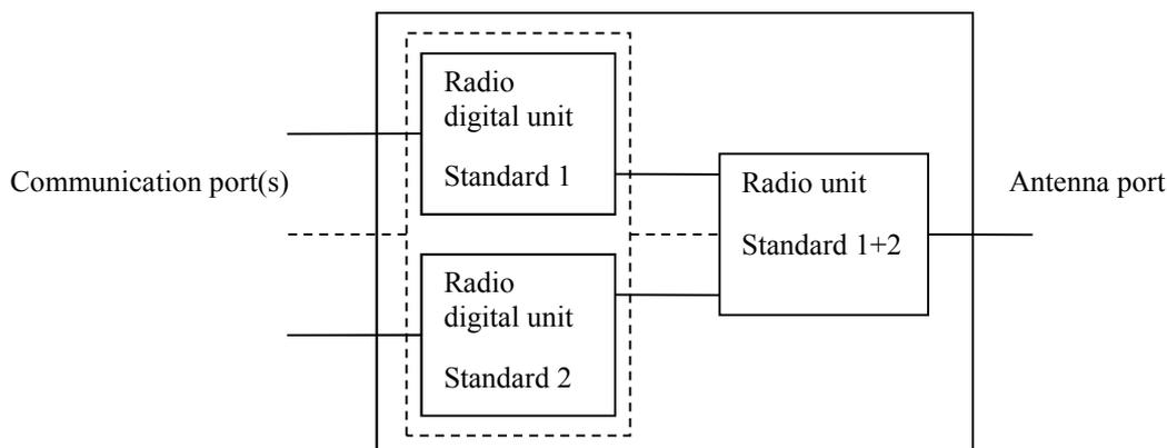
**Figure 2: Multi-standard-radio equipment**
