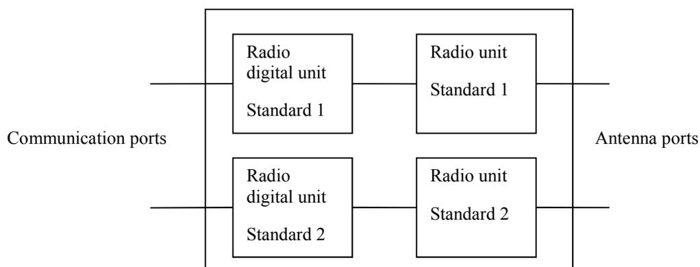
**Figure 1: Multi-radio equipment**
